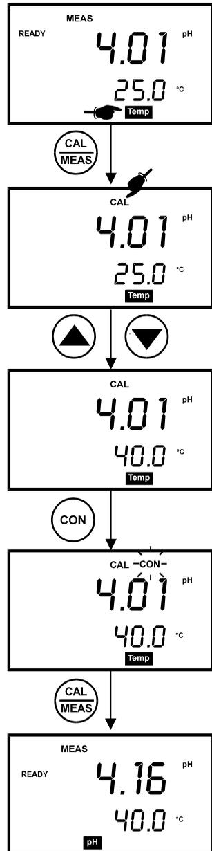
Figure 18: Temperature Calibration
