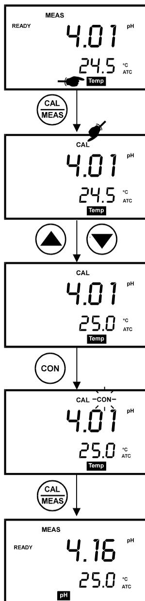
Figure 19: Temperature calibration with temperature probe
