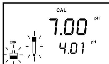
Figure 17: Err message and electrode icon will appear if incorrect buffer are used
