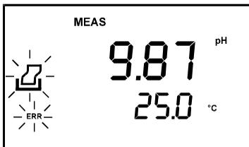
Figure 56 - "Print" and "Err" icons blinking
