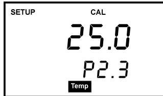
Figure 31: Temperature of the last calibration performed
