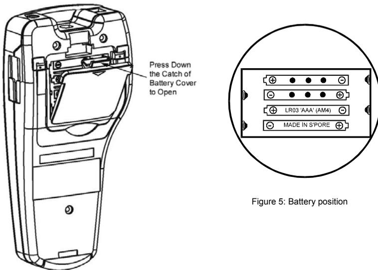
Figure 4: Back panel of meter showing battery compartment
