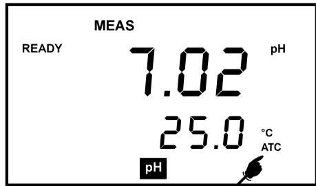
Figure 21: ATC annunciator will light up when connected to temperature probe
