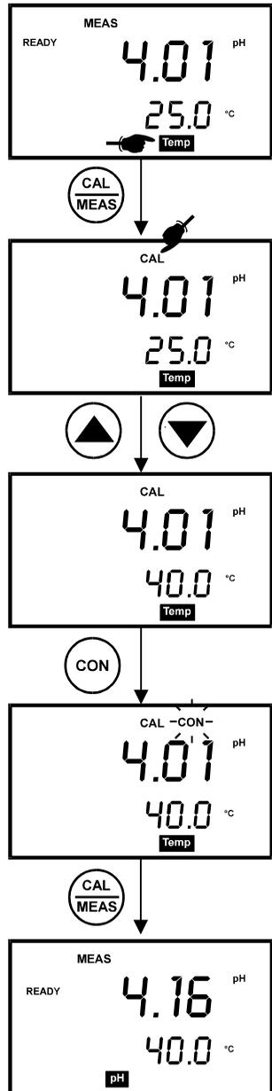
Figure 22: pH measurement using Manual Temperature Compensation
